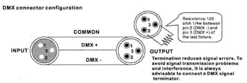
CAUTION Do not allow contact between the common and the fixture's chassis ground. Grounding the common can cause a ground loop, and your fixture may perform erratically. Test cables with an ohm meter to verify correct polarity and to make sure the pins are not grounded or shorted to the shield or each other.
