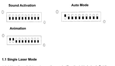
1.1.1 Use dip switch to set operating mode (See the table below). Set the operating mode according to clients' requirement: **SOUND ACTIVE** or
