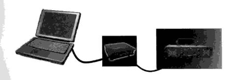
Lighting software like Phoenix, Pangolin and ISHOW can work with laser which has ILDA interface.
