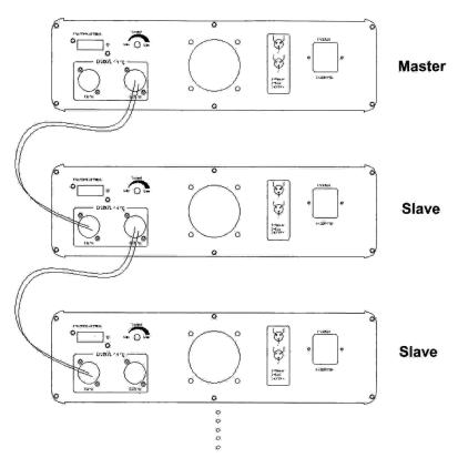
The switching way of Master& Slave synchronous mode
