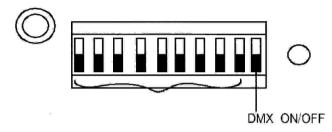
When in DMX mode, the DMX controller controls the laser, and the corresponding function of every channel is shown in attachment. The DMX address code is in the attached address table.
